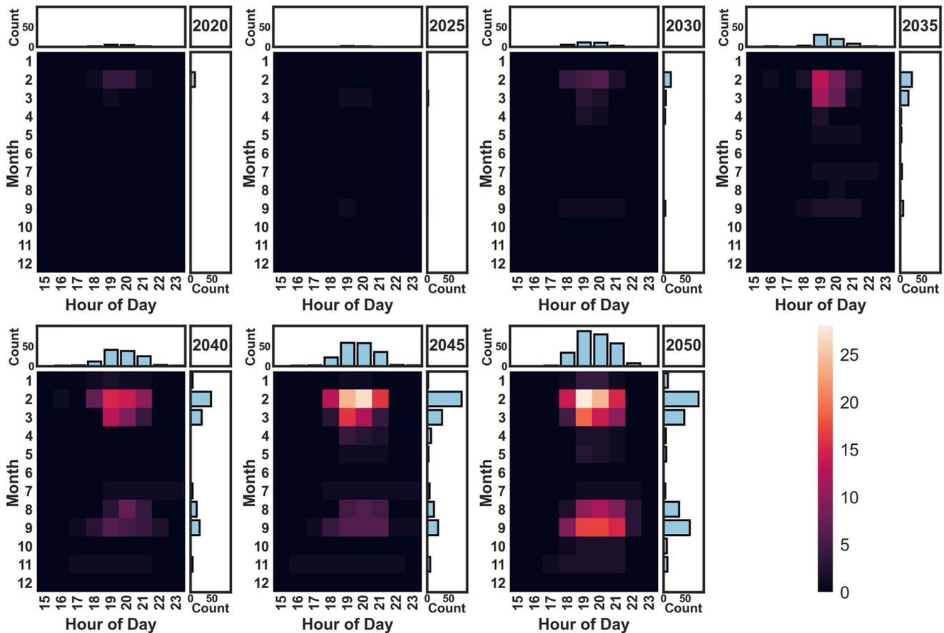
**Figure 8.** Heat maps showing shortfalls on two timescales in the California Independent System Operator system for EV technology pathway. Vertical axes show months of the year, while horizontal axes show evening hours of the day. Although the late winter shortfall events appear more frequently than in late summer, the severity of summer shortfalls was found to be much greater in terms of the total amount of slack generation dispatched.
