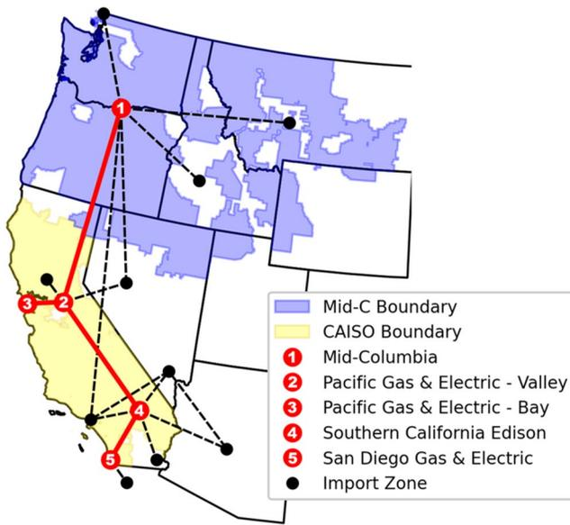
**Figure 1.** System topology of California and West Coast Power Systems model, showing the five modeled zones and boundaries of the two major systems. Power exchanges among modeled zones 2–5 are modeled mechanistically, while all other exchanges are trained on historical data (2008–2012) and modeled statistically.
