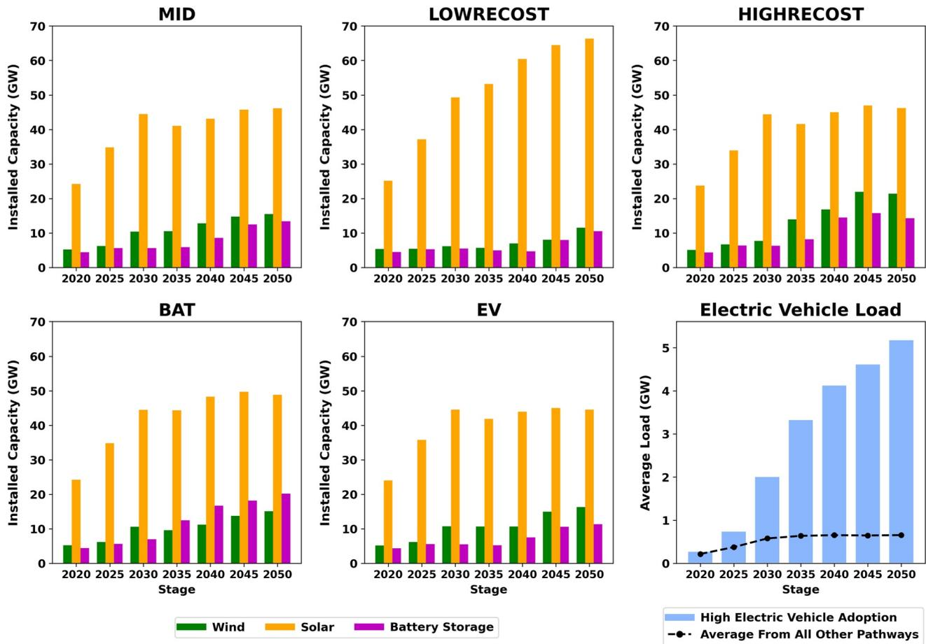
**Figure 2.** Renewable energy additions over time for each technology pathway in the California Independent System Operator (CAISO) system. Additions of wind, solar, and battery storage for each pathway are shown in five of the panels, while the sixth shows the average additional load experienced by the system due to electric vehicle adoption. In this bottom right panel, only the high electric vehicle adoption pathway is significantly different from the others.
